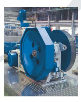
The mechanical briquette presses are made out of a robust welded-steel. The eccentric drive with heavy flywheel operates energy efficient and reliable.
