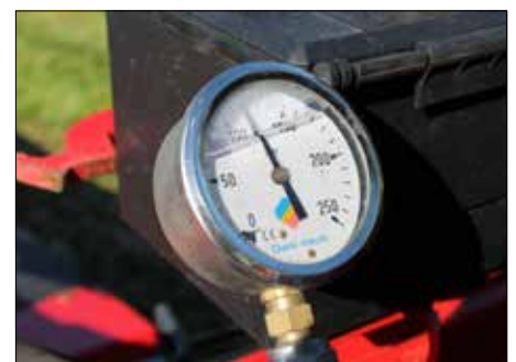
A Manometer shows the ground pressure
