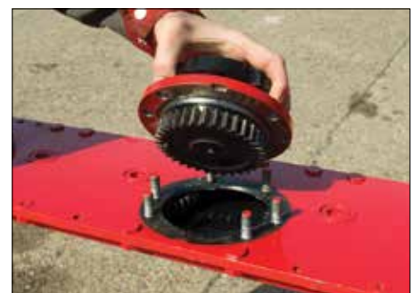
The Top Service design of the cutter bar makes it possible to check and replace a gear wheel or bearing on each disc
