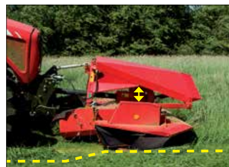
Contour Float - uneven ground following
